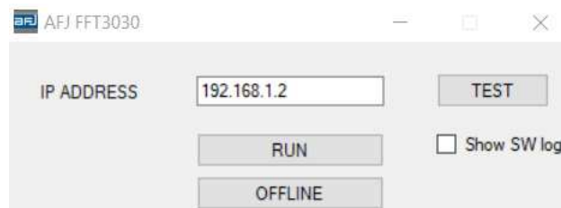
Fig. C.18: FFT 3030 EMI receiver IP address setting
