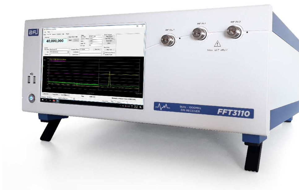
Fig. B.1: AFJ FFT 3110 EMI Receiver
